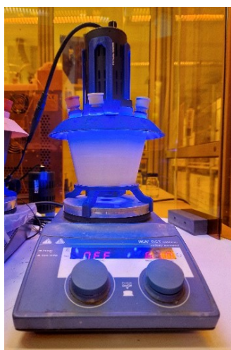
Figure 27. Picture of the assembled Ufo reactor equipped with a Kessil lamp ( \lambda_{em} = 456 \text{ nm} ).
