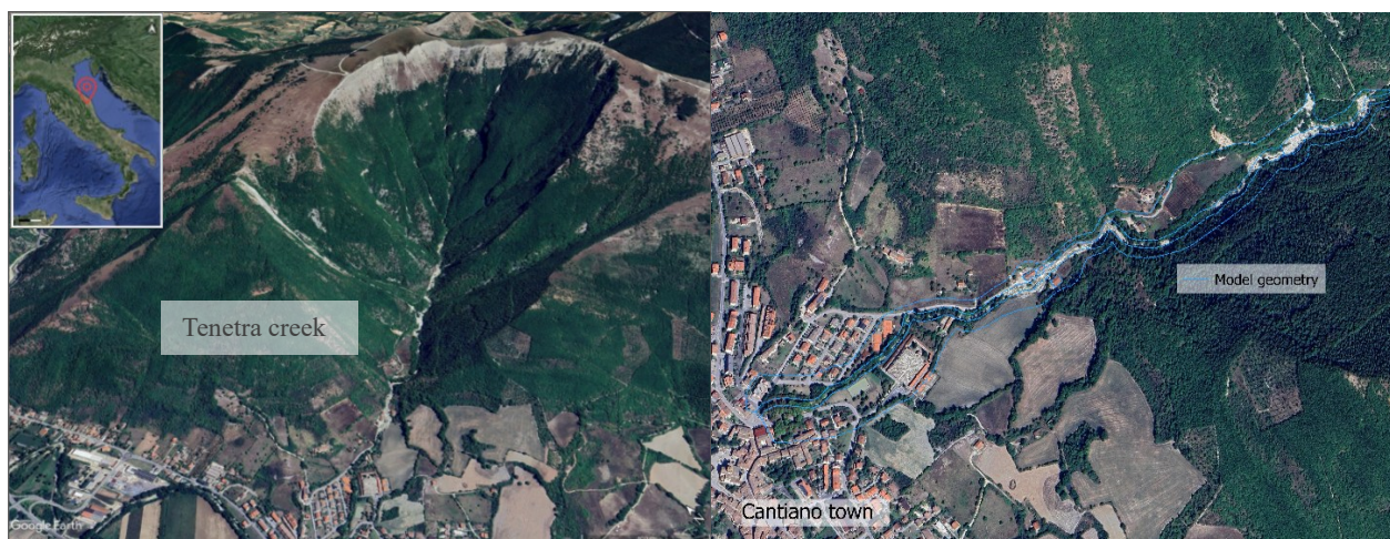
Figure 1 Tenetra river basin on the left: the highest point of the basin is Mount Tenetra, while the town of Cantiano is located at the bottom of the image. On the right, the segment analysed shows the geometry designed in QGIS, used for the construction of the mesh in the numerical model.
