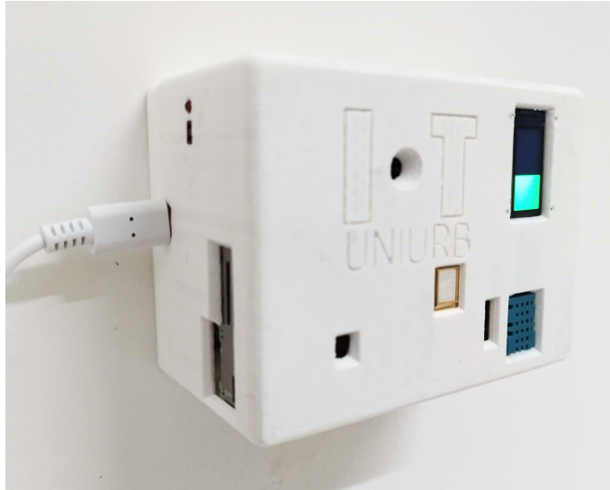
Figure 3.3: Photograph of the actual IoT sensor deployed in a classroom.
