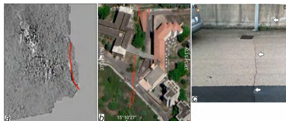
Figure 17. (a) Phase gradient ascending Sentinel-1 interferogram highlighting the southern end of the Acireale Fault (red line). (b) Google Earth image of the surveyed ground ruptures (red lines) in the Capo Mulini site (see Figure 11—coordinates: 37^{\circ}34'50.1''\text{N} – 15^{\circ}10'28.1''\text{E} ). (c) Road pavement asphalt with centimetric ground ruptures (photo March 2019).
