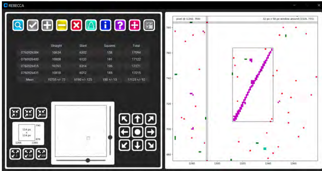
Fig. 14. Example of automated and visual analysis carried out with REBECCA. Left panel: four different matrices corresponding to the peak of the same SEP event are analyzed at once. The mean number of particle tracks in the sets of analyzed cosmic-ray matrices and standard deviations are reported in the bottom row of the table in the figure. Right panel: subregion of a cosmic-ray matrix is shown, after the automated analysis. By default, the last opened matrix is shown. Users can change this behavior by clicking on a different row of the table in the left panel. When dragging the mouse over the shown subregion, the corresponding matrix pixel’s coordinates are shown in the top left corner. When “Select mode” is on, it is possible to draw rectangles around tracks of interest and the corresponding coordinates are reported in the top right corner. A quick guide of REBECCA, explaining the functionalities associated with each button of the interface, is accessible through the “?” button in the main window.
