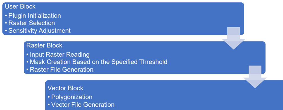
Fig. 3. Schematic representation of the sequence of processes executed on the system side
