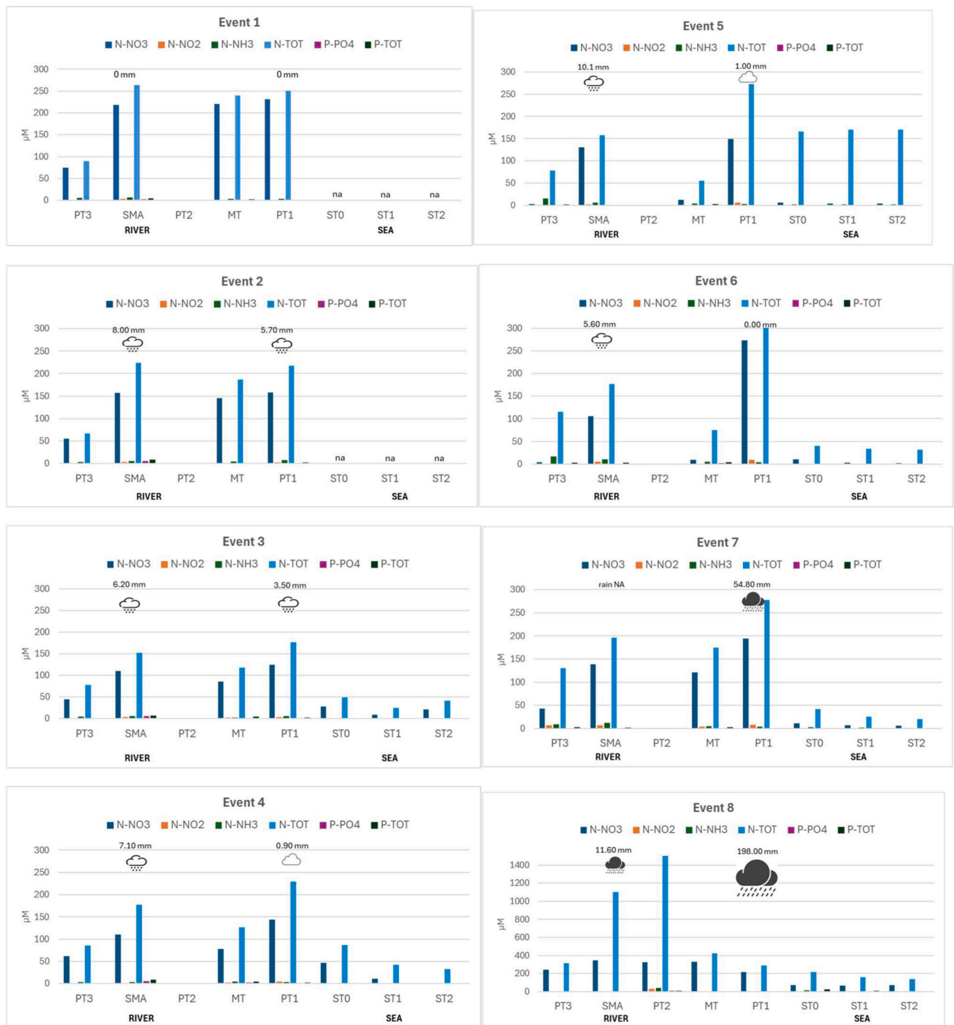
Fig. 4. Concentrations of dissolved inorganic nutrients: nitrite ( \text{NO}_2^- ), nitrate ( \text{NO}_3^- ), ammonia ( \text{NH}_3 ), and inorganic phosphate ( \text{PO}_4^{3-} ), measured in the river basin and adjacent coastal area during eight sampling events conducted under different weather conditions.
