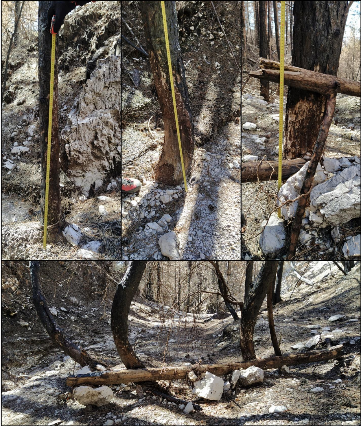
Figure 10 – Photographs showing flow erosional signature on tree stems (i.e. thickness) after the August 24 event. Pictures are taken along the Fosso delle Piscine channel, below the headwater catchment. In this segment of the channel flow thickness reached a maximum height of ~120 cm.
