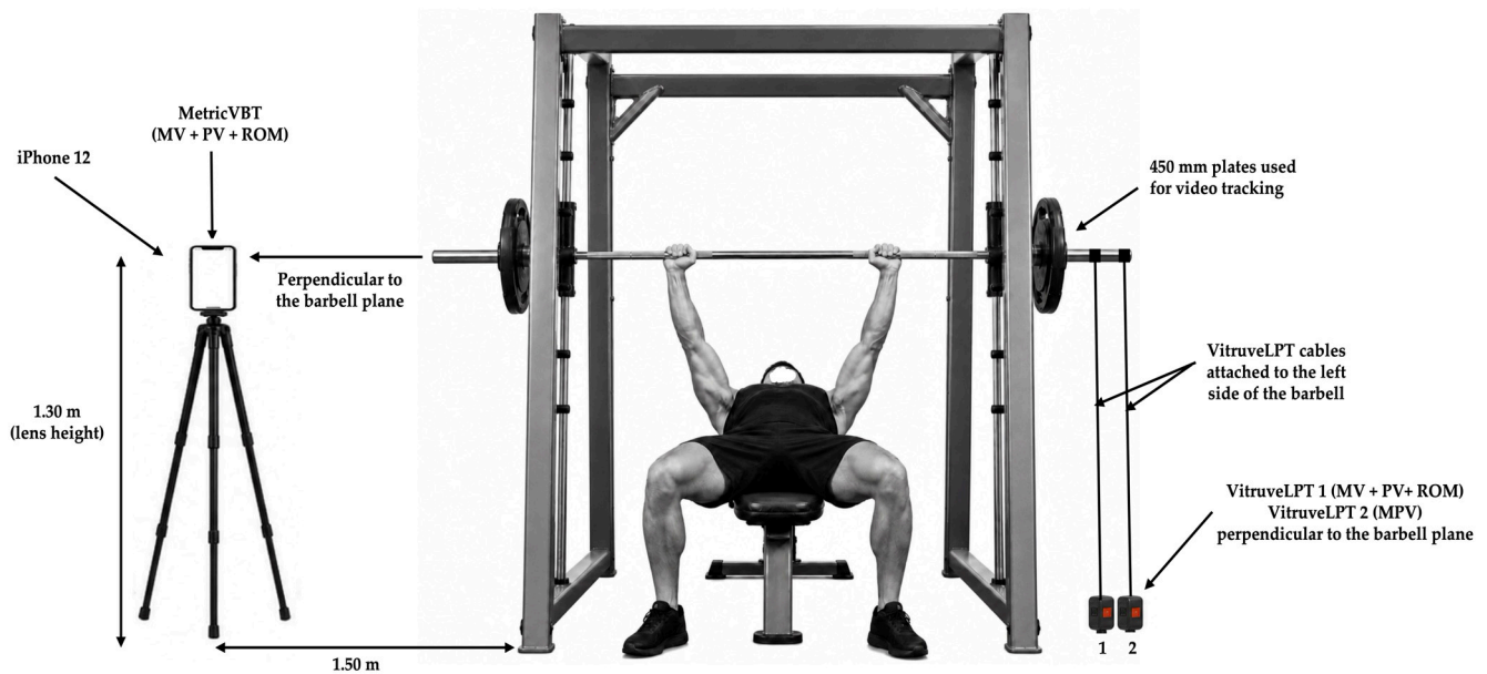
Figure 1. Experimental setup: the MetricVBT app was operated on an iPhone 12 mounted on a tripod positioned 1.50 m laterally to the rack, with the lens set at 1.30 m height and oriented perpendicular to the barbell plane to record mean velocity (MV), peak velocity (PV), and range of motion (ROM). Two Vitruve linear position transducers (VitruveLPT) were placed on the floor on the opposite side of the rack, directly perpendicular to the barbell's right side, to simultaneously record MV, PV, ROM, and mean propulsive velocity (MPV). This graphical illustration was generated with AI assistance (ChatGPT, version 5.5) and subsequently edited by the authors to accurately represent the experimental setup.
