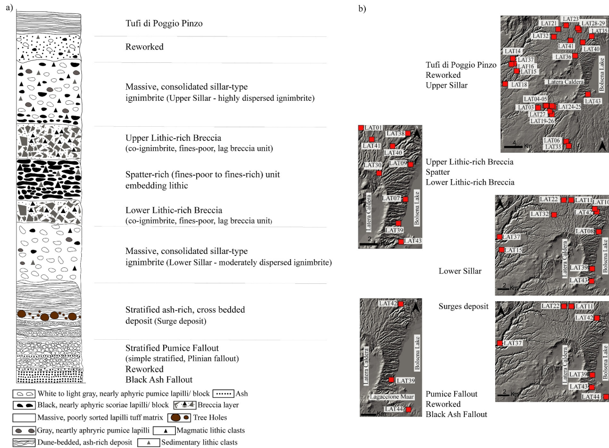
Figure 13. (a) Synthetic depositional sequence representative of the intermediate/distal deposits of the Grotte di Castro-Onano eruption. Not to scale. (b) Location of the sites studied for each deposit. DEM model is derived from Tarquini et al. (2007).
