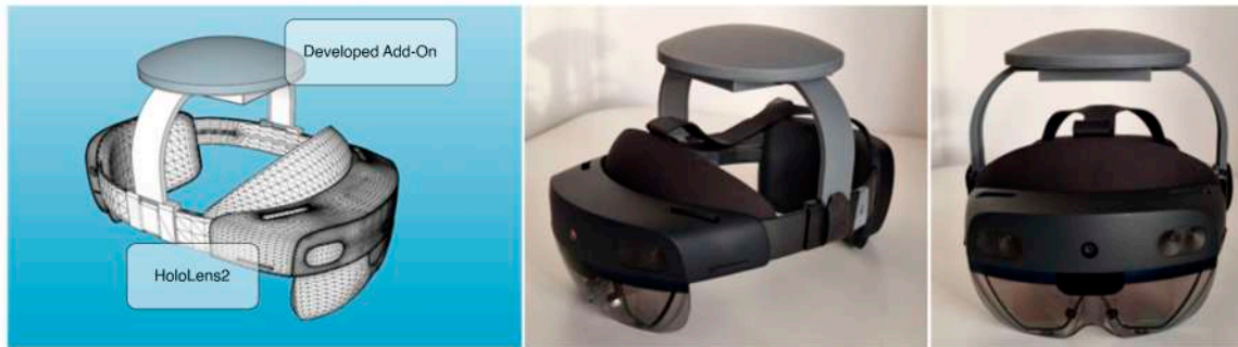
Figure 5. In-house 3D printed prototype of the RTK receiver. The add-on is rigidly attached to the HoloLens 2 device for testing purposes.
