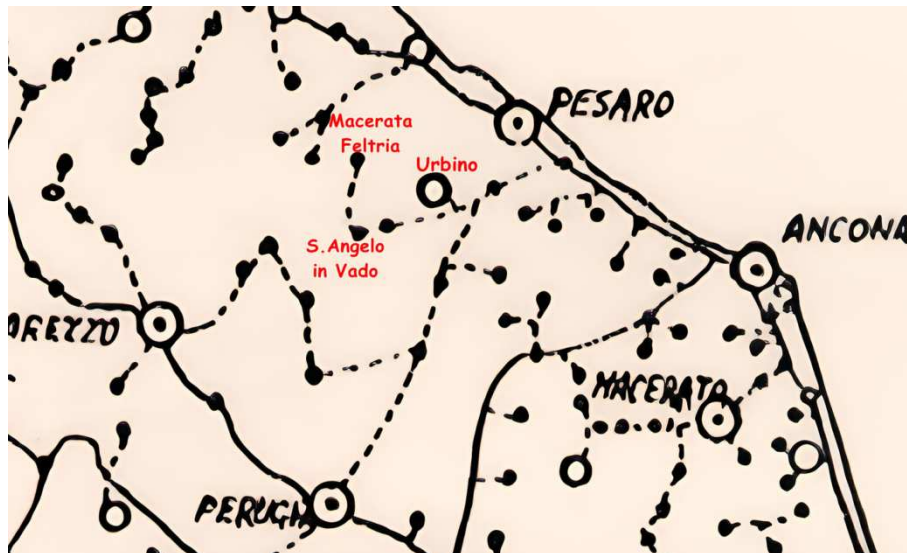
Fig. 30 Detail from the official map Telegrafi italiani. Carta delle linee e degli uffici dello Stato (Rome, January 1878), showing the telegraph lines used by Serpieri in his 1878 telephone experiments: Pesaro–Urbino–Macerata Feltria (118 km), Urbino–Macerata Feltria (56 km), and Urbino–Sant'Angelo in Vado (29 km). Red place-names added by the author for clarity. Sources: Courtesy of TIM Historical Archive, Turin; (Antinori 1963, Tav. I, p. 16)
