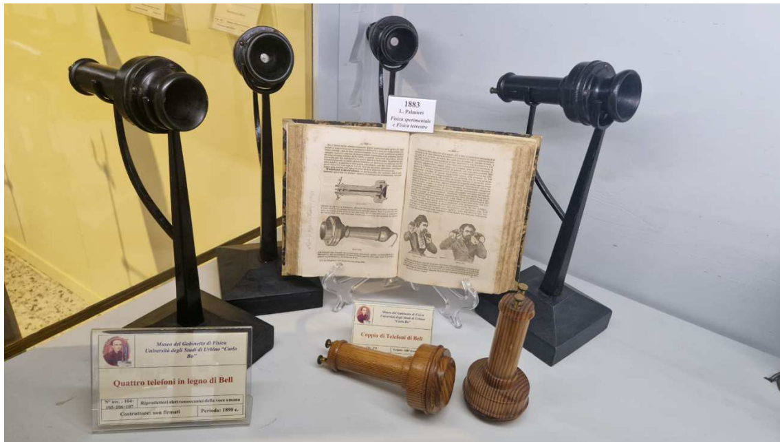
Fig. 29 Set of Bell telephones purchased by Serpieri, now preserved at PLUMST. In the centre, the physics textbook by Luigi Palmieri is open to the section on Bell's apparatus (Palmieri 1883, 352–353). The four black-lacquered instruments on stands are most likely those acquired from the Loescher firm in Turin and used in early 1878 for experiments along the Pesaro–Macerata Feltria telegraph line. Source: PLUMST Collection, University of Urbino Carlo Bo (photo by the author)
