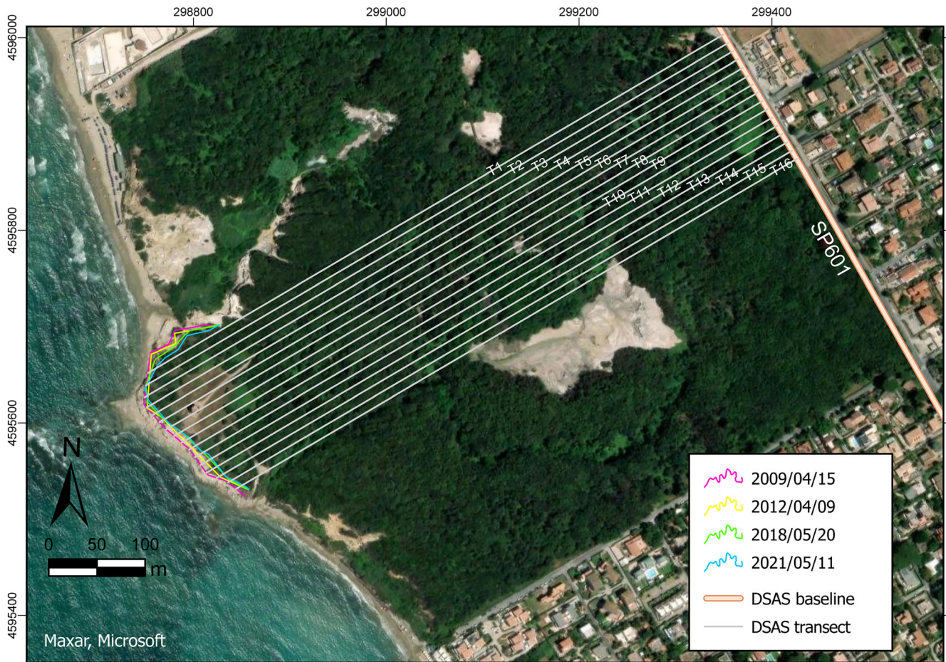
FIGURE 3 The transects (T1-T16) considered in DSAS and the cliff crests reconstructed for 2009, 2012, 2018 and 2009.
