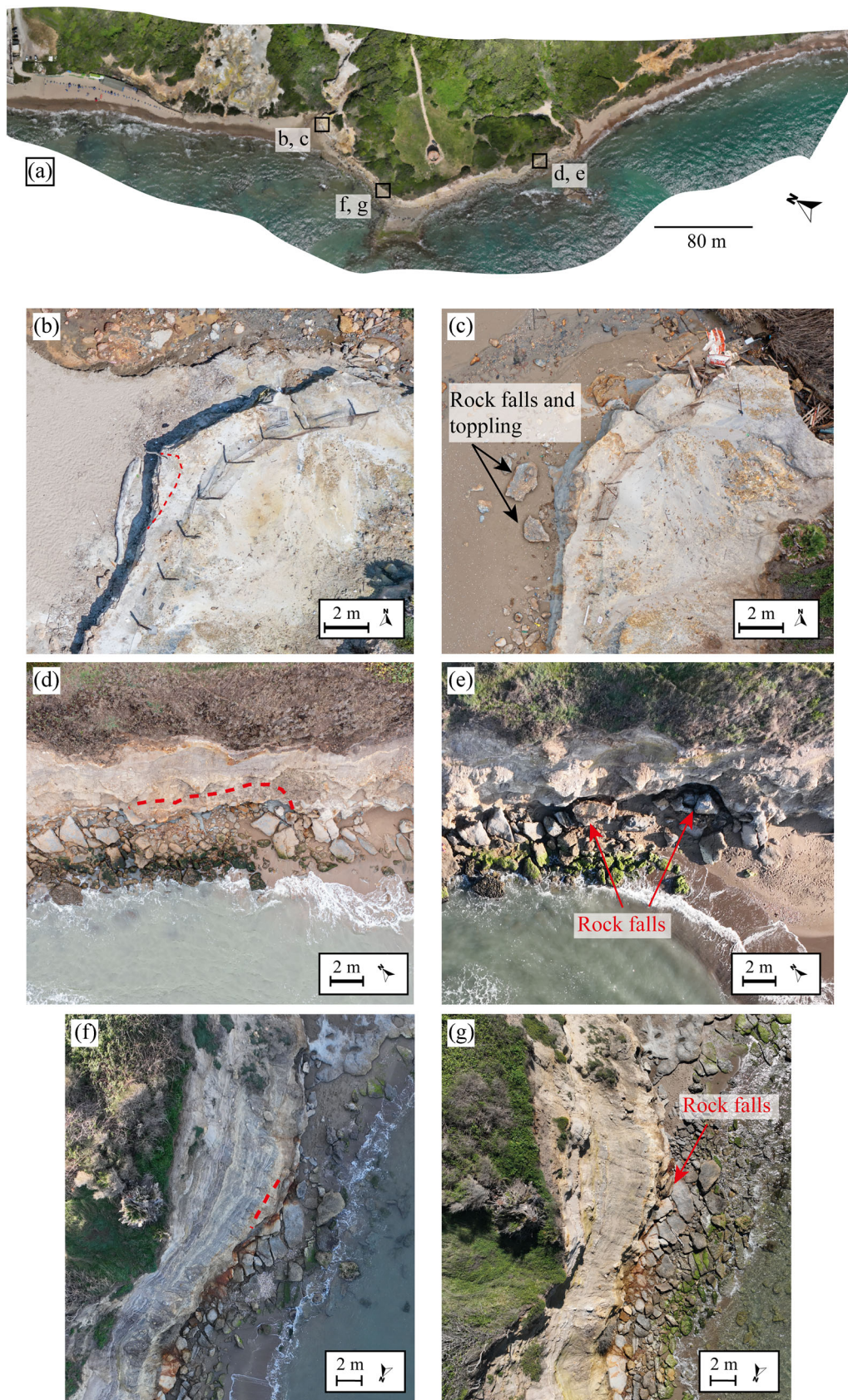
FIGURE 5 Optical multi-temporal analysis of the rocky coastal sector of Tor Caldara reserve. a) Orthophoto-mosaic of the Tor Caldara study area, one of the first survey outputs (F0) made with Agisoft Metashape software. The other images are captured with UAV surveys and are pre- and post-storm events: F0 (b) vs F1 (c), F1 (d) vs F2 (e) and F2 (f) vs F3 (g), with the red dashed lines and arrows indicating the rock falls.
