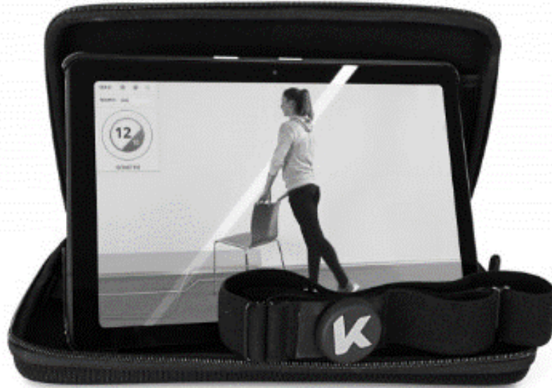
Figure 1. The figure illustrates the technological solution consisting of a tablet (the dedicated software displays video instructions and real-time visual feedback) and a wearable inertial sensor (magnetically attached to an elastic band).
