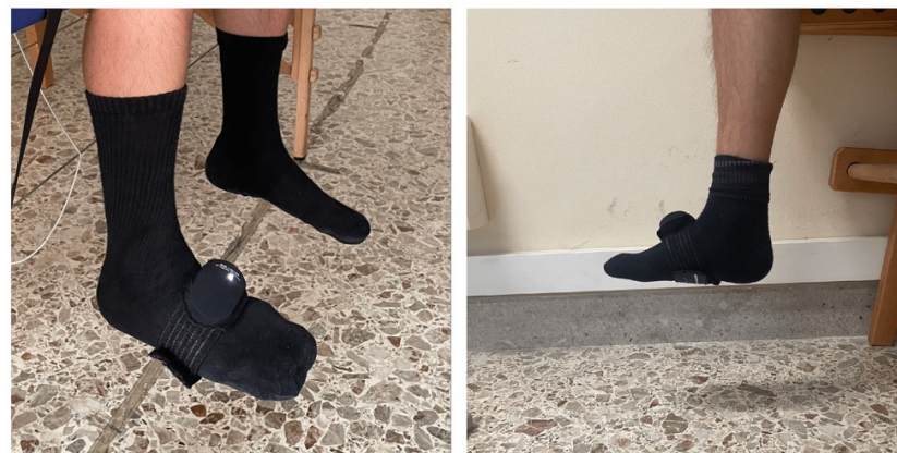
Figure 1. Instrument setting of Beyond Inertial on the ankle joint.
