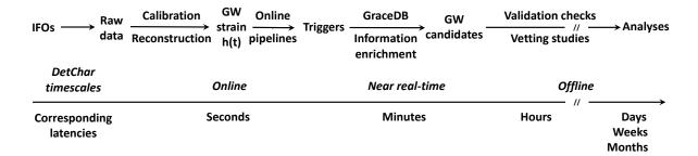
**Figure 5.** Dataflow from the interferometers (labeled "IFOs" on the left) to the offline validation of GW candidates and the completion of the final dataset (right). It focuses on the generation and the vetting of the public alerts that are a key product of the LIGO-Virgo observing runs. It shows the three main timescales at which the Virgo DetChar group operates: online, near real-time and offline (see text for details).
