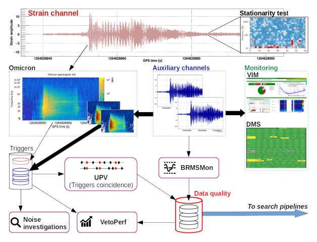
**Figure 3.** Generic workflow of transient noise studies in Virgo, using the full set of DetChar and monitoring tools described in Reference [16].
