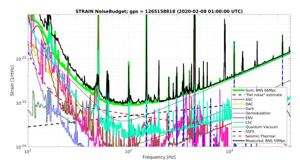
**Figure 6.** Snapshot of the AdV O3 noise budget generated at a time of near best sensitivity of the detector (February  $8^{th}$ , 2020). The different noise sources shown are described in the text. The green line (BNS range: 66 Mpc) represents the sum of these noises: it can be compared to the measured total noise shown in black (BNS range: 59 Mpc).
