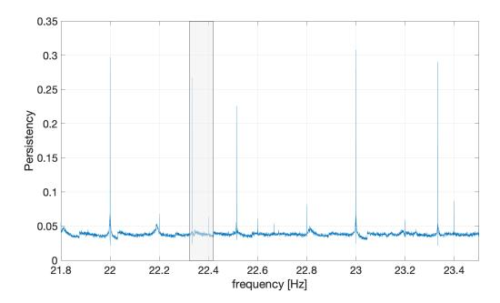
**Figure 17.** Plot of line *persistency* over the frequency band 20 Hz to 30 Hz. The grey box identifies the frequency range covered by a narrow-band search of CW signals from the Vela pulsar in O3a data. The line at 23.333 Hz, which contributed to produce a candidate in the search is clearly visible. In fact, several other lines belonging to the 1 Hz *comb*, both at integer frequencies and shifted by 0.333 Hz, and to a weaker 0.2 Hz-spaced comb, are present.
