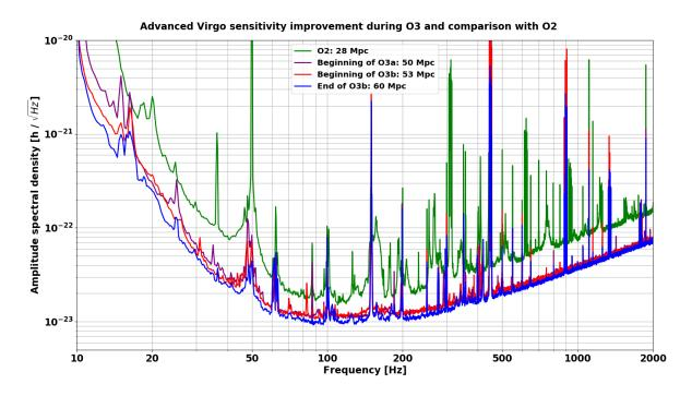
**Figure 8.** Comparison between four sensitivity curves of the AdV detector: during O2 (green trace), at the beginning of O3a (purple), at the beginning of O3b (red) and at the end of O3b (blue). The caption provides the corresponding estimated BNS ranges.
