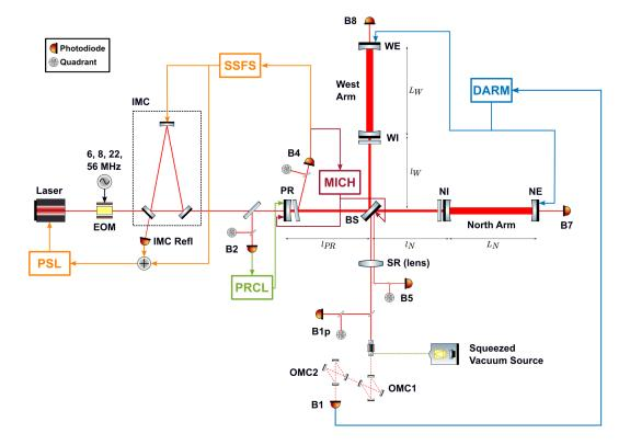
**Figure 2.** Schematics of the AdV configuration during the O3 run (not to scale), showing optics, photodiodes and quadrant photodiodes, such as the main components of the global feedback system used to steer the detector. The suspended optical benches introduced in the text are not represented here. This figure is taken from [31].
