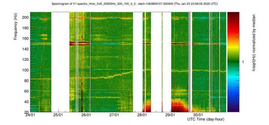
Figure 18. A typical 7-day spectrogram of the h(t) channel, generated by the Spectro tool [16] and allowing the monitoring of a wandering spectral line whose main frequency was first stable around 83 Hz before increasing up to around 100 Hz in about a day.
