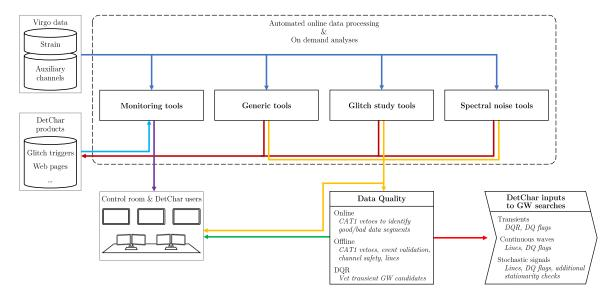
**Figure 1.** Flowchart of the Virgo DetChar tools and monitors described in [16]. The corresponding data quality (in short "DQ") products are used to monitor the detector and as inputs to GW searches.
